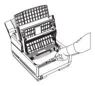
6. Pull out the paper cassette. If any of the paper in the paper cassette is damaged, remove and replace it.
